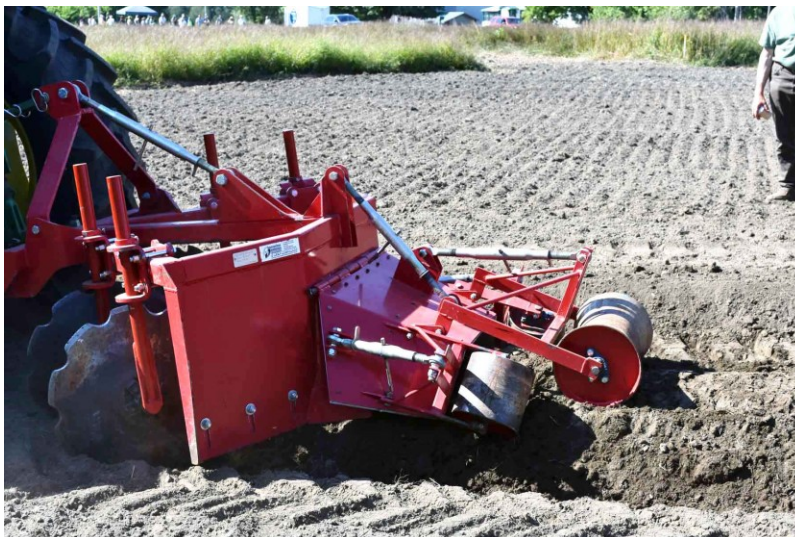
Cultivator designed in Quebec to develop raised outplant beds for seedlings
